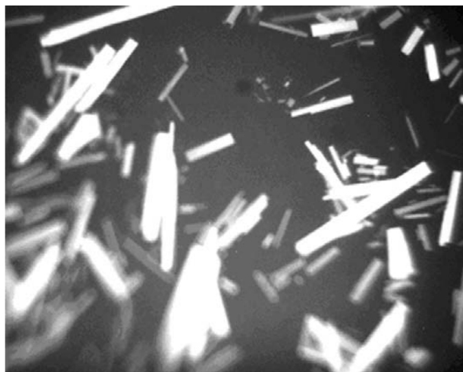
Figure 4 Glucose isomerase crystals imaged by ultraviolet fluorescence using the epi-fluorescence geometry. The crystals are in a hanging drop on a quartz cover slip in a Linbro plate.
